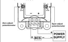
positive terminal, connect the negative power supply lead to the negative terminal of the BCS 4-20 mA input. Last, connect the (-) negative terminal on the CXLdp to the (+) positive BCS input.
