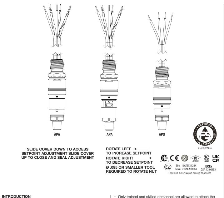
The APS and APA pressure switch have 316 stainless steel housing and process connections. The APS has a factory fixed setpoint which cannot be changed in the field. The APA is field adjustable and can easily be adjusted by following the instructions in the diaphragm above.
