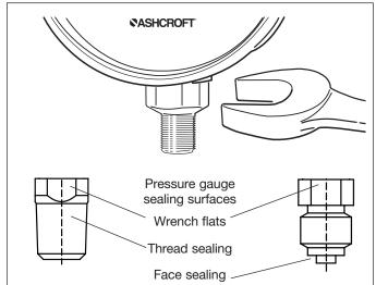
After installation, pull up the blue cap on the fill/vent plug to the full open position. Opening the vent plug will relieve internal pressure changes in the gauge case that otherwise would have been induced by environmental changes in pressure and/or temperature. Without being vented this change in internal pressure could adversely affect the accuracy of the gauge. If liquid filled, only open vent plugs when the plug is oriented in the vertical position.
